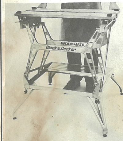
5. Always make sure that each leg locks into its extended position. Ensure adjustable feet for "sawhorse" position do not prevent the legs from fully locking. This will ensure the safe use of the Workmate at this upper working height.
