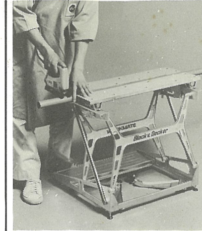
6. Sawing tubular pieces is easy when they are held horizontally in the specially designed V-grooves running along the face of the vise jaws.
