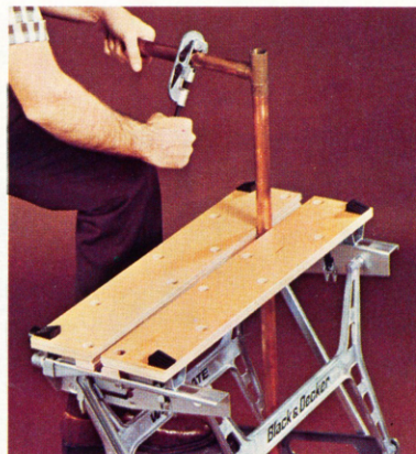
Grooved vise jaws allow vertical grip on pipe and tubing.
