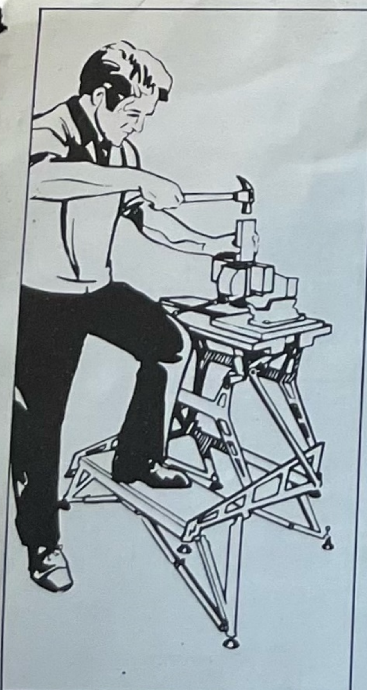
A metal working vice can be used with the Workmate—simply mount it on a wooden board, screwed to a batten and clamp the batten between the vice bars.
