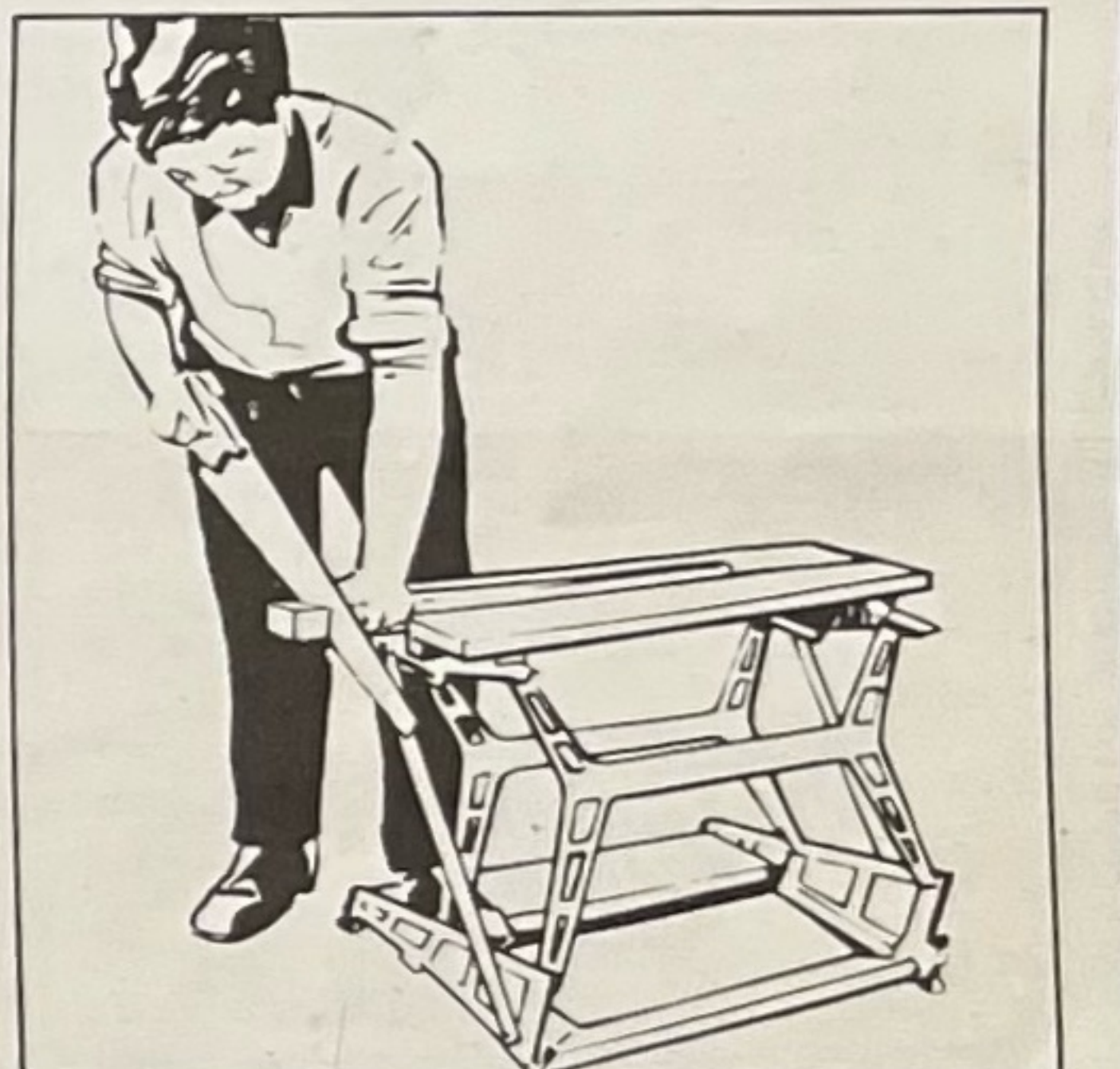
Sawing. Tapered or parallel workpieces can be securely clamped between the vice bars for safe accurate sawing.
