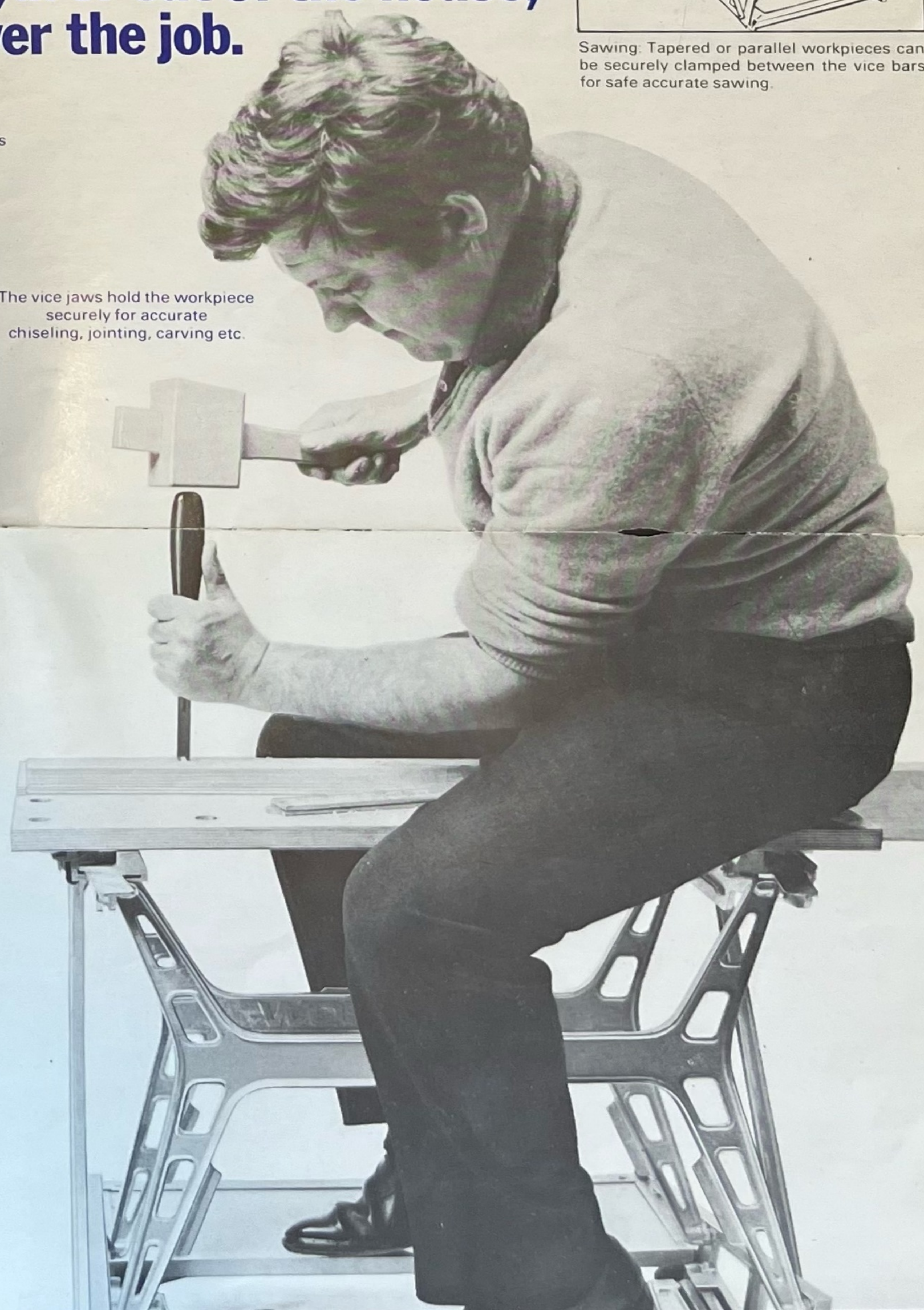
Saw panels up to 8' x 4". You can hold even the thinnest panels with all your weight, and they cut much better being supported right along the cutting line.
