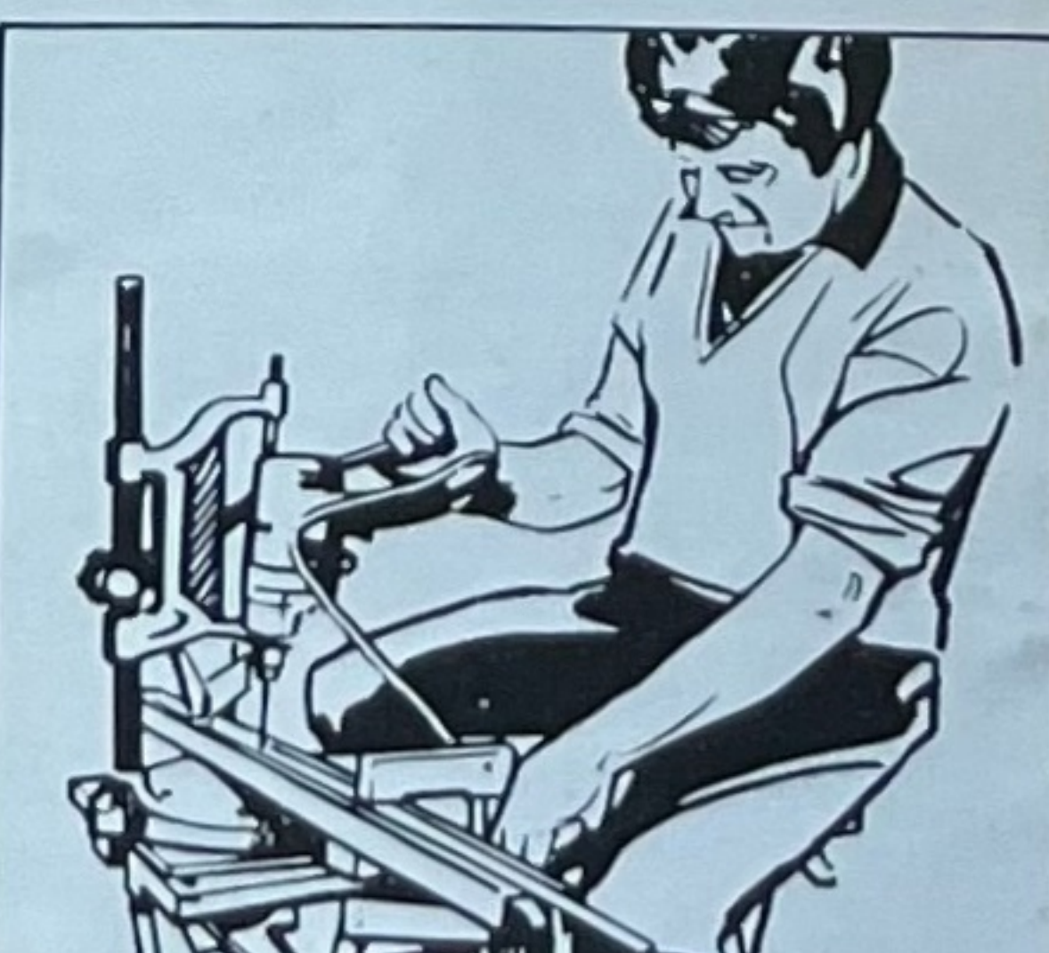
Power tools such as a circular saw, vertical drill stand, woodworking lathe, can be clamped within the vice jaws using a wooden board screwed to a batten.
